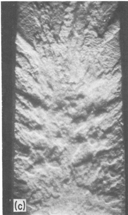
Figure 2 Macroscopic fatigue fracture surface appearance associated with different moisture levels. (a) 0% r.h.; (b) 23% r.h.; (c) 50% r.h.; (d) 100% r.h.
