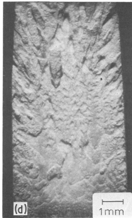
Figure 2 Macroscopic fatigue fracture surface appearance associated with different moisture levels. (a) 0% r.h.; (b) 23% r.h.; (c) 50% r.h.; (d) 100% r.h.
